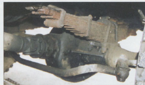
Details of front wheel drive axle on 4x4 chassis. Cardan shaft output diving rear-mounted water pump is shown on the top left picture.
