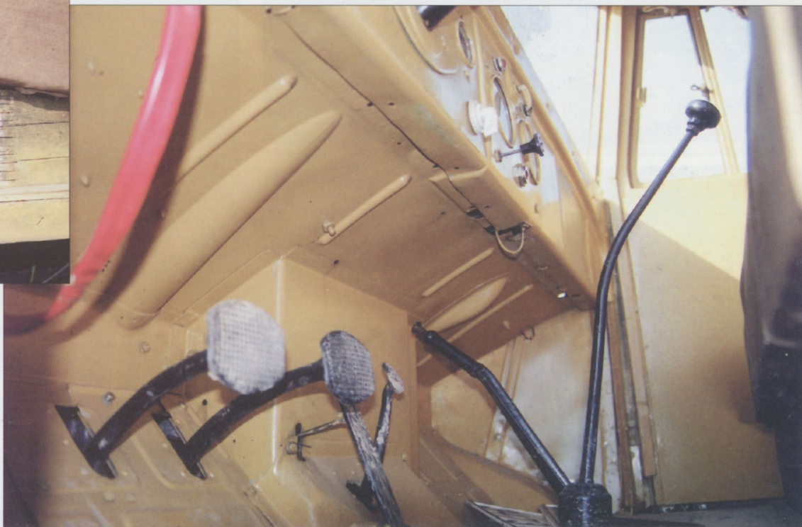
Driver's compartment of Blitz A/p Crash Tender includes original Blitz instrument panel, steering wheel and break, clutch and throttle pedals.
