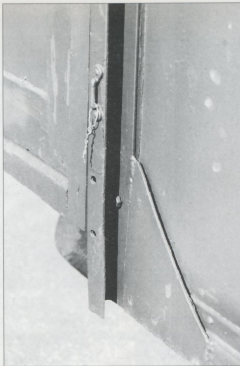
House body details. From top to bottom, from right to left: rear door lock and handle, rear door frame reinforcing, rear door upper hinge and ventilation inlet covers, jerrycan carrier, tool box, side door step, roof access ladder step on rear and front wall of the body.
