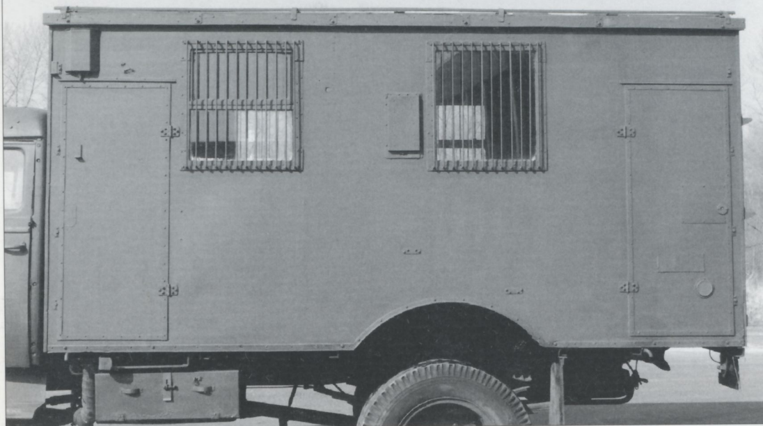
Side view of standard multi-purpose house type body (LC/Koffer). Note that front and rear side windows are different.
