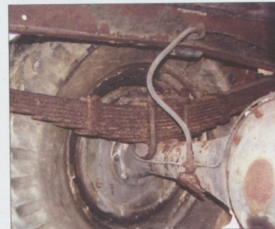
Two typical differential housings were used on Blitz. Bottom right pictures show original banjo-type axle, on the bottom left pictures there is later modification used also on 4x4 variants.
