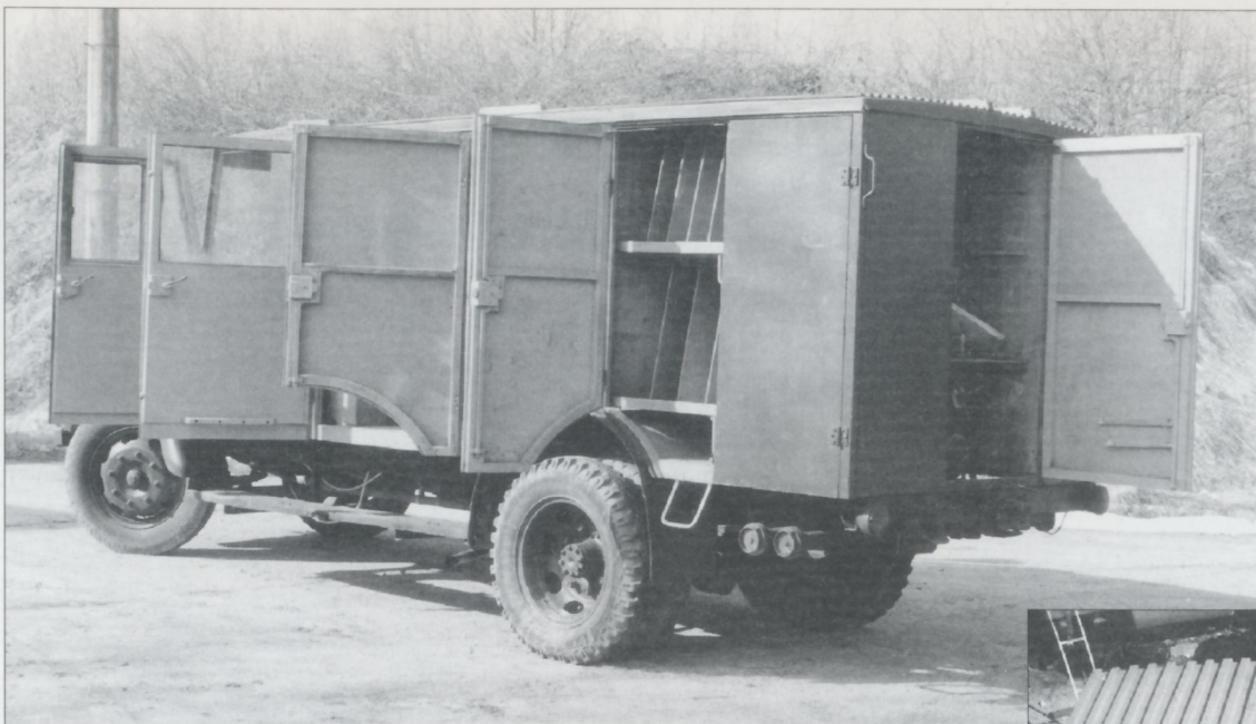
The A/p Crash Tender with all door opened. It is no more clear what equipment was fastened on the cab roof, covered with in all it's length with wooden beams.
